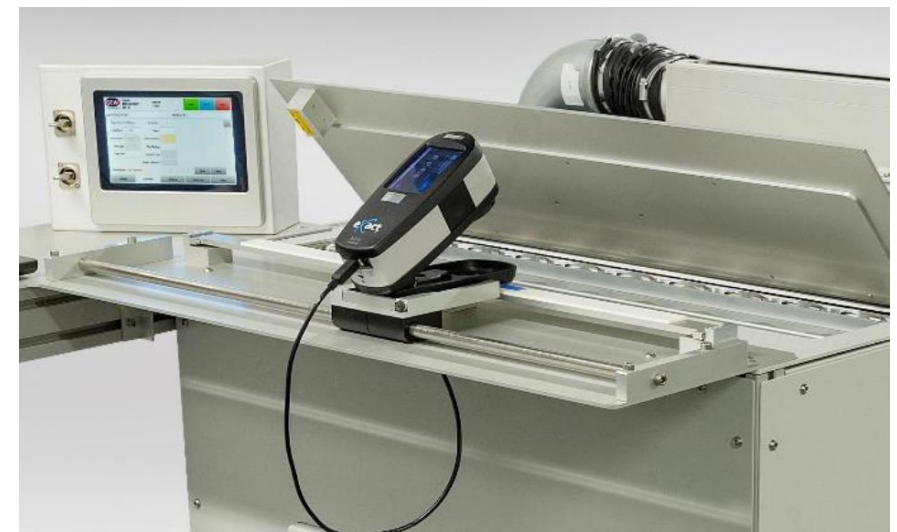
Compact Cassette Laboratory Unit: 1- Cassette adaptor housing. 2- Sample carrier & access hatch. 3- Densitometer, mounting slider & guide rule. 4- GEW Touchscreen 2 HMI. 5- Control panel.
